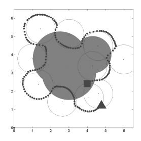
Fig. 9. Vehicle path plot of boundary represented by three intersecting circles. The local circle controller uses a radius of 0.8m with a vehicle speed of 0.15m/s. Square is the starting point and triangle is the ending point. The axes are measured in meters.
